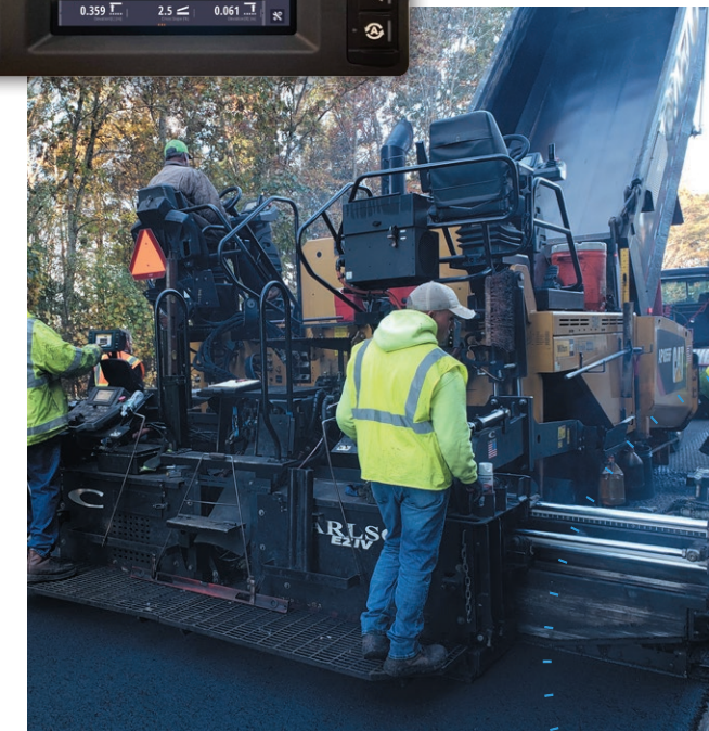
The Trimble Roadworks 2D display features tactile keypads for use in the field
