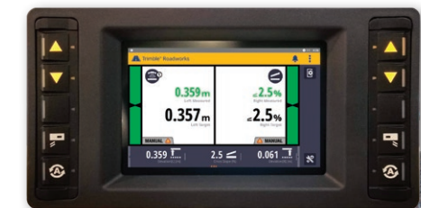
The Trimble Roadworks 2D display features tactile keypads for use in the field
